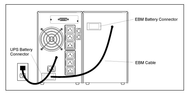
Figure 12. EBM Connections
